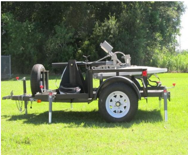
Note: Auto-Acquire antenna stowed and ready to be moved.
