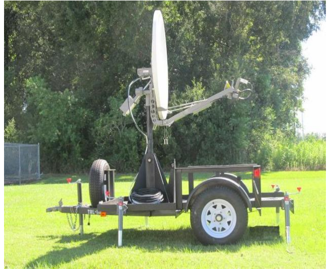
Note: Auto-Acquire antenna fully deployed
